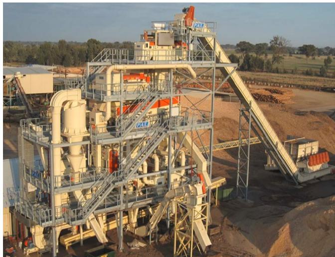
The Cleaning Tower machine was installed new on site some years ago to process recycled wood into a raw material for particleboard. The timber comes from old pallets, crates and furniture offcuts. The timber scraps are shredded into chips, then run through the Cleaning Tower. The Cleaning Tower removes non-wood matter such as metal (ferrous and non-ferrous), plastic and stones as the recycled material 'falls' down the five storey high Cleaning Tower machine.
